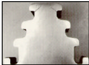
Figure 1. Cracking in the blade-fit area of an HP rotor
