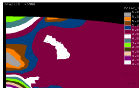
Figure 2: Creep stress contour plots at seam-weld
